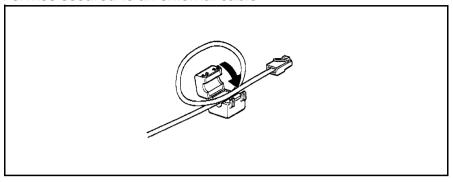
The ferrites are secured to the appropriate cable with plastic enclosure clips. Ty wraps are added to the cable loop.
